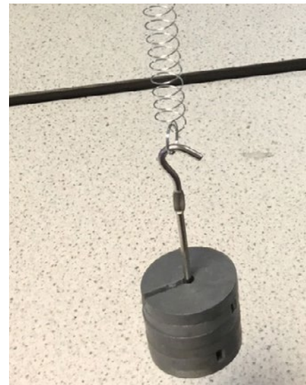
Mass hanger with masses attached to spring suspended from clamp stand
