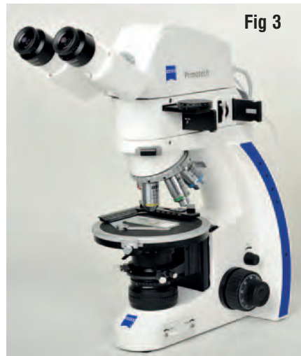
A modern entry-level polarising microscope with digital integral camera. This equates broadly with Hooke's compound microscope. The lighting is now integral within the base of the stand. The microscope can be used both in reflected-light mode (as for Hooke's microscope) or in transmitted-light mode
