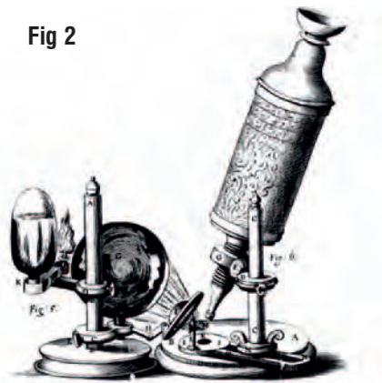
The early microscopes of Leeuwenhoek and Hooke. Many of the components found on a modern microscope (light, condenser, objective, bodytube, eyepiece) can be seen on Hooke's microscope
