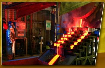
The pouring of gold bars is the final step in a long process. For each gramme of gold extracted from the ore, a tonne of ore must be processed.
