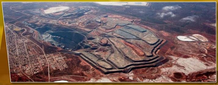
The Super Pit at Kalgoorlie, Western Australia, is 3.5 km long and almost 600 m deep. It produces about 20 tonnes of gold each year, plus 20 million tonnes of spoil. The town has grown to meet the edge of the mine site.
