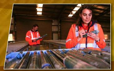
Core samples are analysed for their gold content. Gold is present as gold telluride (AuTe<sub>2</sub>) but, in the ore, just one atom in a million is gold.
