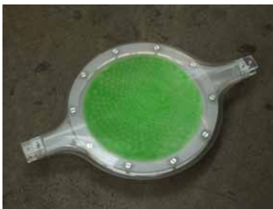
Figure 2 A biophotovoltaic solar panel prototype, and an exploded view showing how it is constructed.
