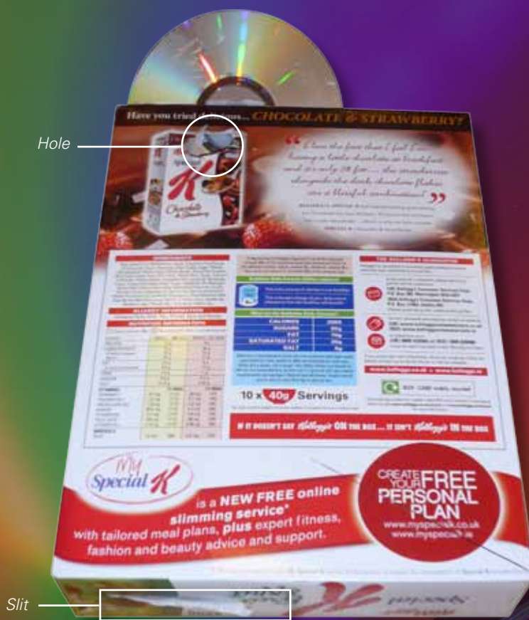
The cereal box spectroscope
