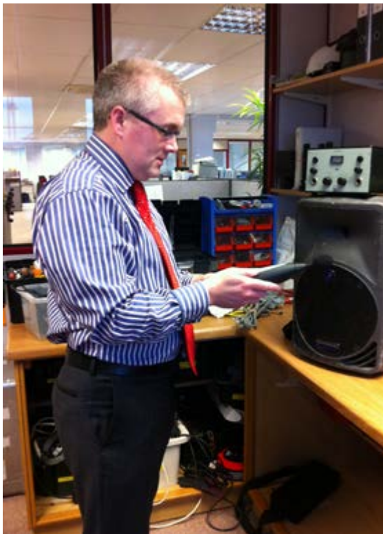
Nick Treby preparing to measure the acoustic performance of a room
