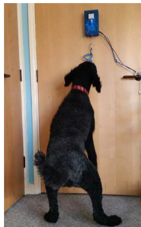
The canine alarm (left), and how it is activated by a dog
