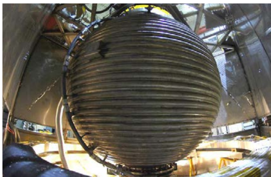
Figure 7 This 3 m diameter sphere contains molten sodium, a metal. When set spinning, electric currents may be produced, resulting in a magnetic field. But will it be similar to the Earth's?
