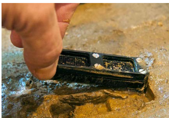
An iChip used for picking up marine sediment in the search for new antibiotics
