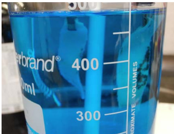
The electroless copper plating bath
