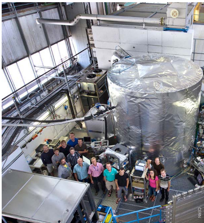
Figure 6 The CLOUD experiment at CERN. Will high-energy protons, fired into the tank, cause clouds to form?
