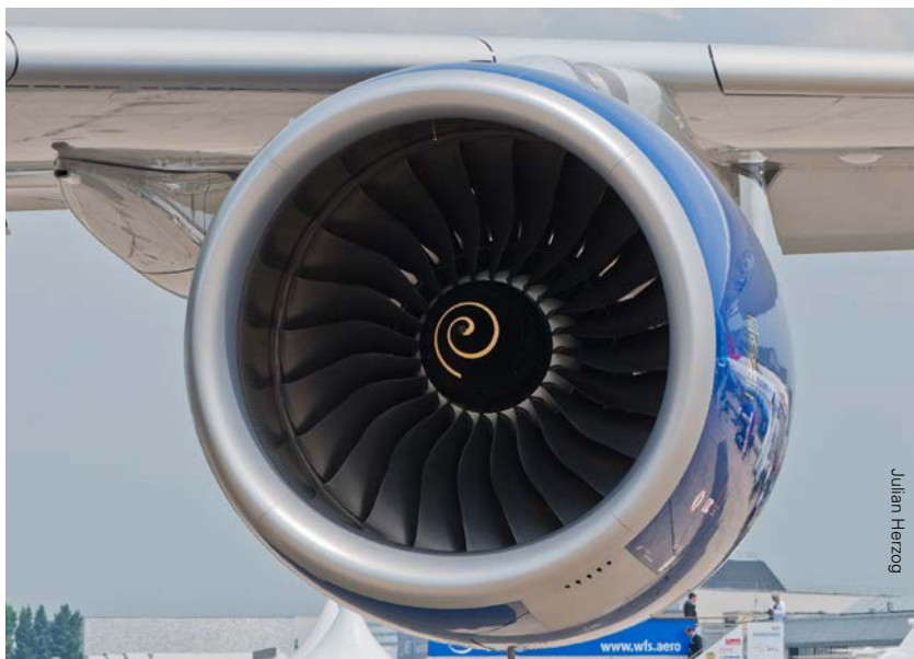
A single jet engine like this can generate a thrust force of 400 000 N.
