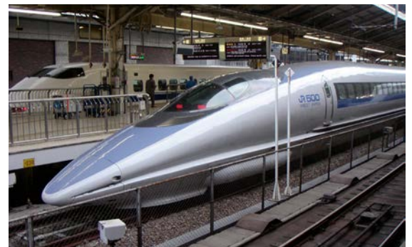
The beak of the kingfisher gave engineers insight into high-speed train design.
