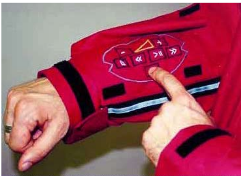
Pressure-sensitive gloves for an astronaut and iPod controls built into the fabric of your jacket – two uses for QTC.
