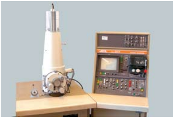
The tall microscope has controls to allow the operator to position the specimen in the electron beam. Images appear on the monitor screen.
