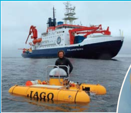
JAGO communicates with its 'mother-ship' by underwater telephone and VHF radio.
