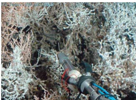
Jago's probe measures oxygen levels in a coral bed.
