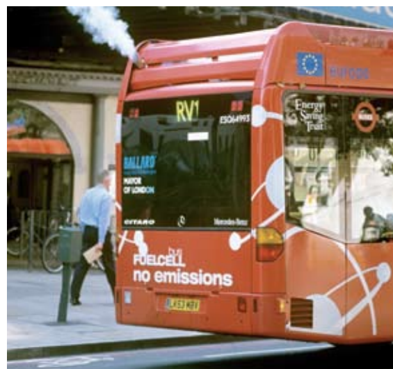
This London bus is powered by hydrogen. You can see steam emerging from the exhaust (top left); this results from the oxidation of hydrogen in the polymer-based fuel cells.
