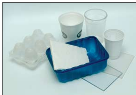
How polymers are processed can make big differences to their properties. All of these items are made from polystyrene.
