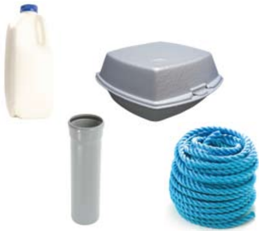
Polymers from different families: milk bottle (polyethylene), fast-food container (polystyrene), pipe (PVC) and rope (nylon).
