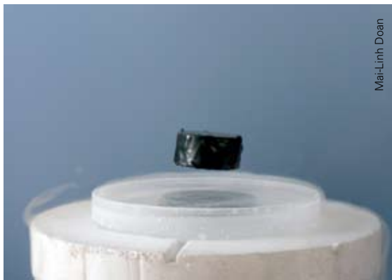
A small magnet levitates above a superconducting electromagnet. Liquid nitrogen is used to cool the superconductor.
