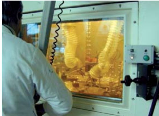
A technician manipulates radioactive materials using remote handling tools; he is protected by lead glass.
