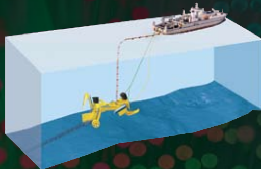
The cable-laying machine is dragged slowly across the seabed, laying the fibre optic cable as it goes.
