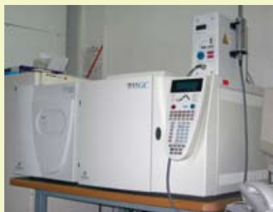
A GC-MS machine, closed and open. The chromatography takes place in the oven on the right; molecules are detected by the mass spectrometer on the left.
