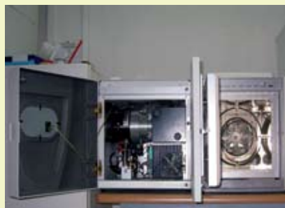
A GC-MS machine, closed and open. The chromatography takes place in the oven on the right; molecules are detected by the mass spectrometer on the left.
