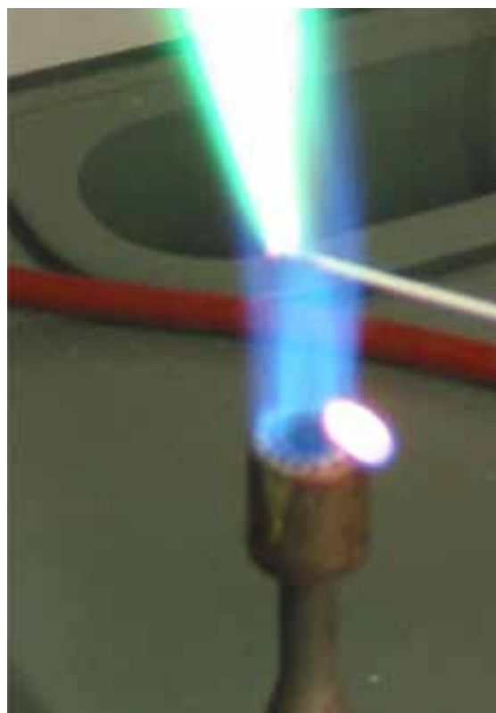
A flame test on copper sulfate gives a characteristic coloured flame.
