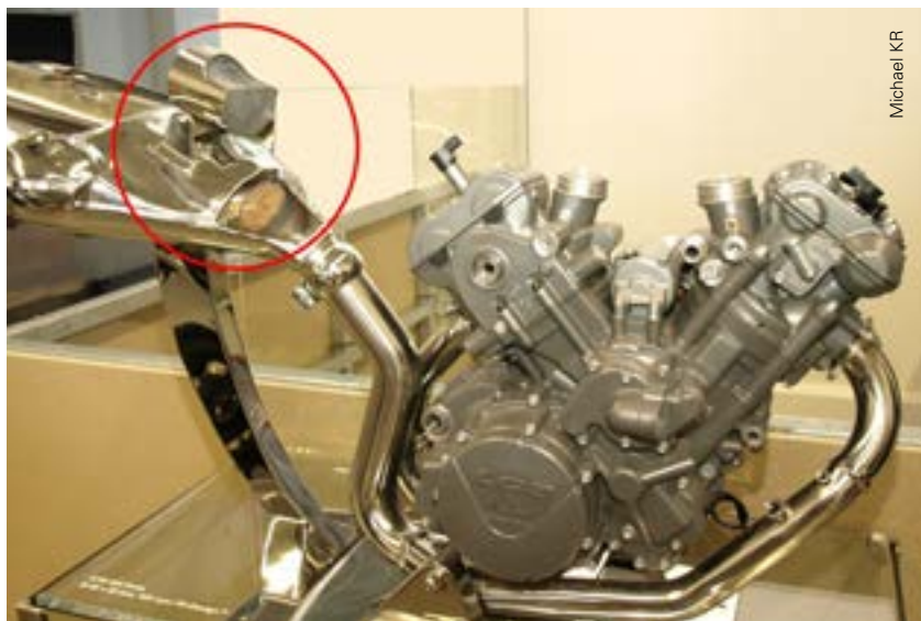
The engine from a KTM 990 Super Duke motorbike, showing the catalytic converter
