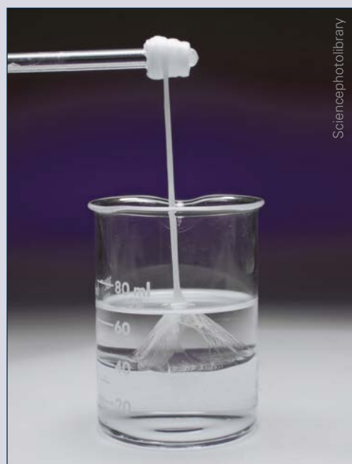
The nylon rope trick is used to demonstrate making nylon in the classroom
