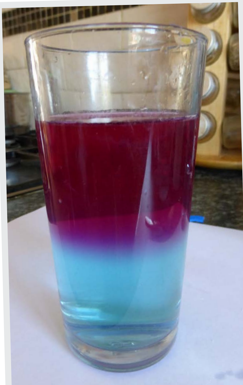
Salt and fresh water form layers which are surprisingly stable – they will remain like this for hours.
