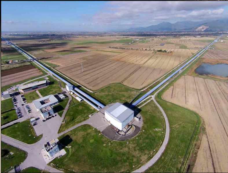
Europe has a gravitational wave lab near Pisa, Italy. You can see the two long arms of the interferometer.
