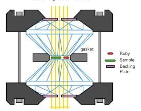
A diamond anvil cell; the sample is held between two diamonds; there is also a ruby which is used to indicate the pressure.
