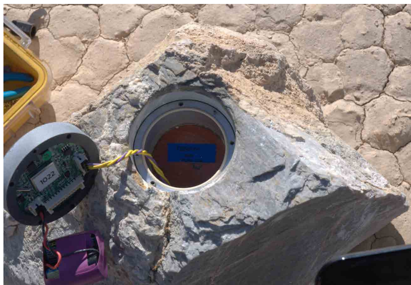
A GPS receiver being installed in a rock
