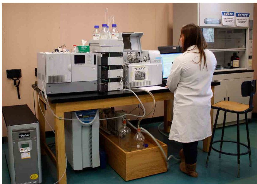
A liquid chromatography-mass spectrometry machine being used to test samples.
