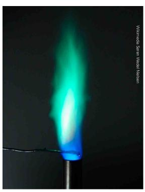
Flame tests can be used to find out which metal is in a sample but not how much – it is a qualitative test. A green flame indicates copper is present.
