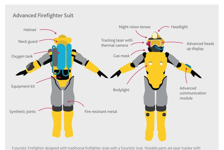
thermal camera, Advanced Heads Up Display, Head and Body Lights, Communication Module, Traditional Firefighter Neck guard and Helmet, and Gas Mask With Oxygen Cylinder
