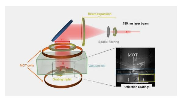
The GMOT coils generate a magnetic field changing in space which increases the probability of atoms drifting further away from the centre of the vacuum cell (trap) to absorb and re-emit red photons from the split laser beam. Thanks to this solution, when an atom moves away from the centre of the trap, its atomic resonance is shifted closer to the laser light frequency, so the atom becomes more likely to get a photon 'punch' towards the centre of the trap.
