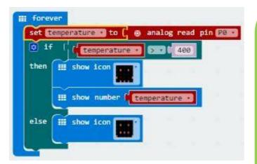
In this example the micro:bit will tell us when the room is too cold by showing the frowny face. As you hold the thermistor the temperature increases and the smiley face will light up letting you know the room is warmer.
