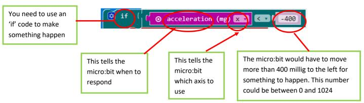
You will need to put this code in a 'forever' loop and you will also need to add lines of code to tell the micro:bit what to do when it is tilted to the left and what to do when it is not.
