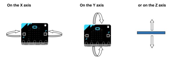
The accelerometer can be coded from the input keyboard where you can decide which axis you want to use.
