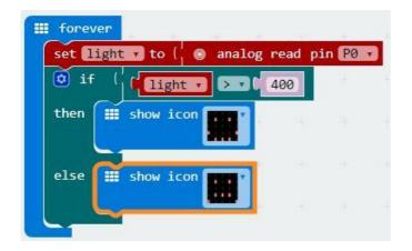
In this example the micro:bit will tell us when it is above a set light level by showing a smiley face. If you cover the LDR the frowny face appears to show us the light level has dropped.
