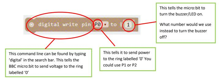
You will need to work out what input you want to use to make your buzzer sound or LED light otherwise they would be on all the time. You will also need to ensure you have a line of code which turns the buzzer/LED off at some point.
