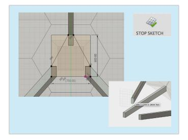
Activate the top component by clicking on the white circle. Then create a new component named Secondary Mirror.
