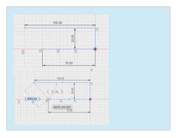
Create another line, this time from the top of the previous line. Make a line going outwards by 100mm, at a right angle to the vertical line.
