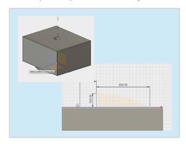
Create, Revolve. Select the previous sketch (this is the profile), click on axis and select the green axis pointing upwards (Tip: Try hiding Bodies in the Browser to help select the right axis). Make sure the operation is set to New Body.
