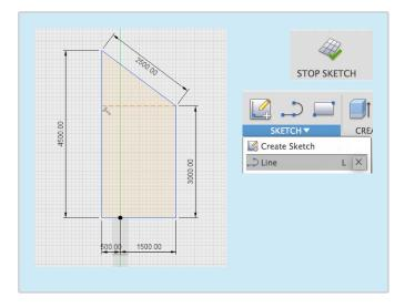
Create a new sketch on the plane shown above, the view cube should be on the Right view. Tip: Click on the right side of the view cube then select the plane.
