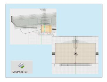
6 Create a new sketch on the side plane shown above. Complete the following sketch using the line and dimension tools. The path should start from the center of the spacecraft bus.
