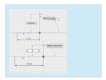
Draw a new line, this time connect the two ends or the horizontal line together. Click one end and then the other to create the line.
