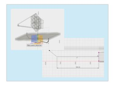
8 Create, Sweep. Keep type on Single Path. Select the profile which is the circle. Then select the path being the first line sketch. Make sure that chain selection is turned on. Then mirror the new body using the mirror tool and plane shown.
