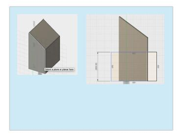
8 Create, Mirror the previous extrusion onto the other side of the module. Change pattern type to features and select the last extrusion in the timeline. Then select the mirror plane going down the center of the module.
