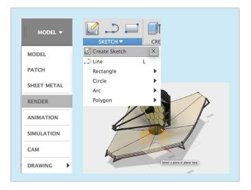
Create, Extrude, half of the previous sketch creating a semi circle wall. Change the direction to symmetric and extrude both sides as shown.
