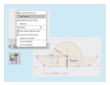
This time, instead of using the extrude tool, try using the revolve tool. Go to create and then revolve. The revolve tool will ask for profiles you want to revolve. Select one half of the sketch as shown above.
