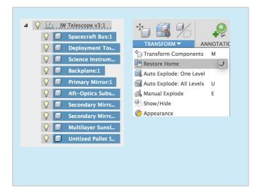
Instead of auto explode, try manually exploding parts by selecting the component you want to explode, then choose the direction you'd like it to move in. Use the slider to change the scale.
