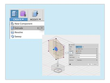
6 Create a sketch on the front of the Backplane as shown. Create a Circumscribed Polygon with 6 side and a diameter of 650mm in the middle of the Backplane.
