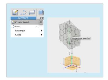
4 Construct, Offset Plane. Offset a plane 1200mm away from the Primary Mirror.
