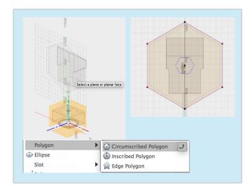
8 Create, Pattern, Rectangular Pattern. Change pattern type to bodies, Select the hexagonal body. Click direction and select the green axis. Pull the arrow upwards. Distance 2600mm and quantity 3.
