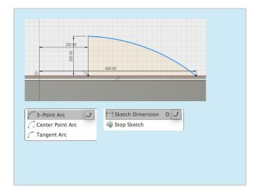
Create a new sketch on the plane shown above. Complete the following sketch on top of the body, sketch 250mm away from the origin. Then create a line going upwards by 200mm. Finally draw another line along the top of the spacecraft outwards by 800mm.
