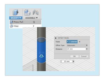
Repeat the same process. Extrude the top of the cylinder by 1000mm upwards, change the operation to new body.
