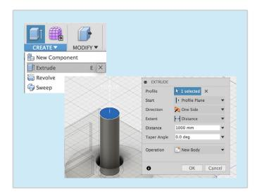
8 Repeat the process, Modify, Press Pull, Click on the top cylinder and offset by a distance of 50mm.
