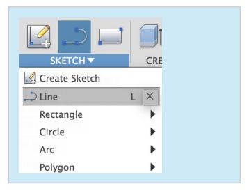
8 To dimension the line type in how long you want to make it. Make the line 75mm going along the red axis. Press enter on your keyboard to create the line. You can change the dimension by click on it.
