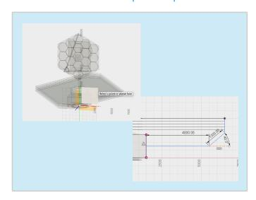
4 Create, Sweep. Keep type on Single Path. Select the profile which is the circle. Then select the path being the first line sketch. Make sure that chain selection is turned on.
