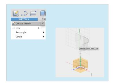
4 Create, Extrude the hexagon outwards by 300mm with a taper angle of 35 degrees.
