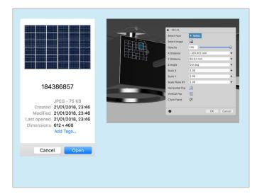
Decals can be added to a face. Click on the blue box with a D to add a Decal. Select the face you'd like to apply a decal to.
