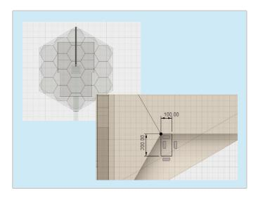
Complete the Sketch by creating a 2 point rectangle from the bottom corner of the Aft-Optics Subsystem, 200mm high by 100mm wide. Make sure the first point is on the corner. Stop sketch when completed.
