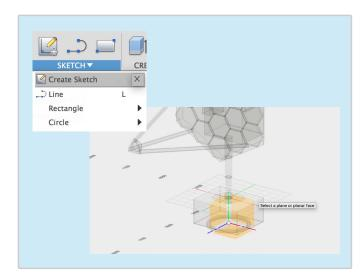
4 Complete the following sketch using the Line and dimension tool. Once completed stop sketch. Start by drawing a line upwards by 9500mm and another line along the red axis by 6500mm.
