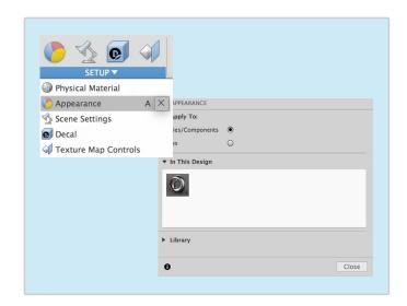
More appearances can be downloaded using the arrow. Right click on an appearance in the 'in this design' box to edit a material. Here you can change the colour of the material, increase the roughness etc.
