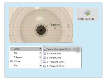
Create a new sketch on the top face of the body (notice its ghosted as we're working on a new component).
