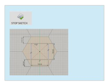
Create a new sketch on the front of the primary mirror, the view cube should be on the Front view.
