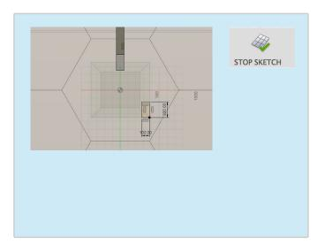
In the browser open the secondary mirror support component. Go into Construction and show plane 1 using the lightbulb. Create a new sketch on this plane.
