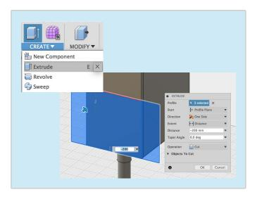
6 Create a sketch on the side of the module (Shown above). Create a 2 point rectangle 2000mm high making sure the rectangle is wider than the module. Stop Sketch.
