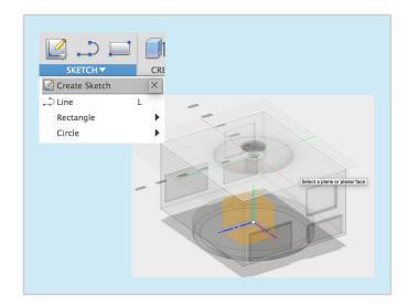
4 Create, Extrude the circle upwards by 1250mm.
