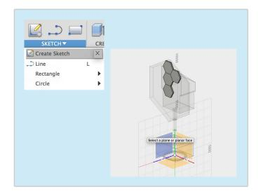
Create, Pattern, Circular Pattern. Change the Pattern Type to Bodies. Select the bodies shown above. Click on axis and select the line created on the previous sketch. Change the quantity from 3 to 6.
