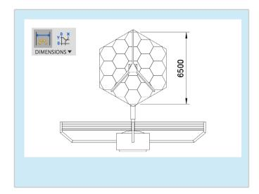
8 Create a new base view by going to Drawing view, Base View. This time change the orientation to a Isometric View and increase the scale to 1:75.
