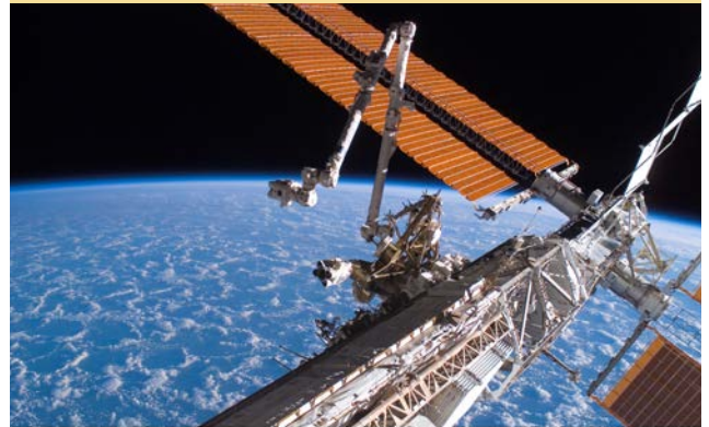
The Canadarm2 (center) and solar array panel wings on the International Space Station.
