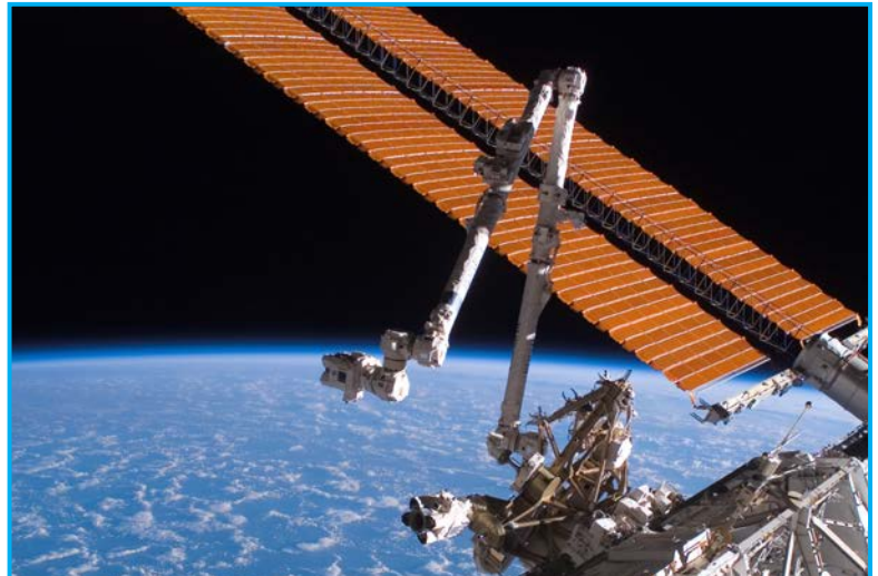
Canadarm2 and its end effector as seen from the ISS.
