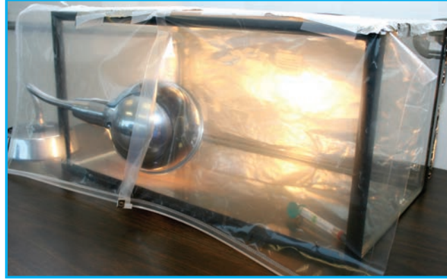
Image 2: Incubator made from a 10-gallon aquarium with closed plastic cover.
