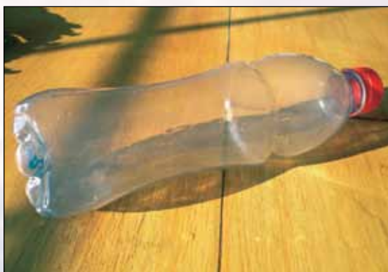
A cloud has formed inside the bottle. This is not the same as condensation as it is not on the inside surface of the bottle, but in the air inside.
