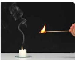
A class discussion can lead students into understanding that in a glass wick candle, the liquid wax is soaked up the wick. On blowing out their candle, they will see a plume of 'white smoke' coming from the wick for a short while. This is condensed wax, and can be lit again with a flame – students will enjoy this trick of relighting the candle from the 'smoke', and a flame can jump several centimetres down to the wick.
