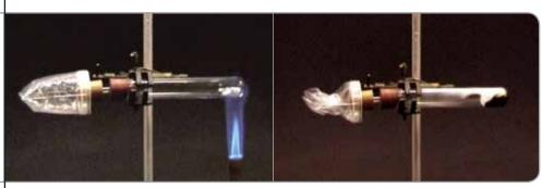
On heating, there is enough oxygen in the tube to start a reaction and further oxygen from the bag pushes in. Once the reaction gets going, the Bunsen can be removed and the bag is seen to collapse as the magnesium continues to react.
