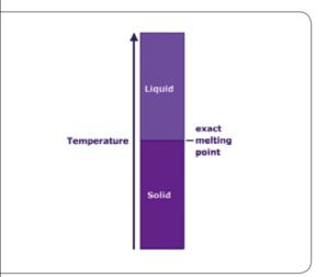
This diagram from the Stuff and Substance e-resources can be used to reinforce the idea of a melting point. Students can also be asked about solidifying – what would happen if liquid wax at 80 °C is allowed to cool? The liquid wax would start to solidify at 64 °C – though at this stage it would be acceptable to argue this will be when the temperature falls just below the melting point.
