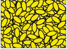
As well as showing the movement of the particles, the representations also indicate the 'grip' that particles have for each other: the thicker the line, the greater the grip and the higher the melting point.
