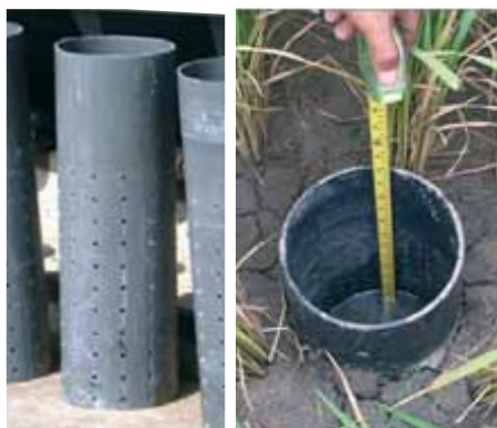
A magic pipe is a simple device which allows farmers to irrigate rice only when it is needed, saving about 50% over traditional paddy field methods.
