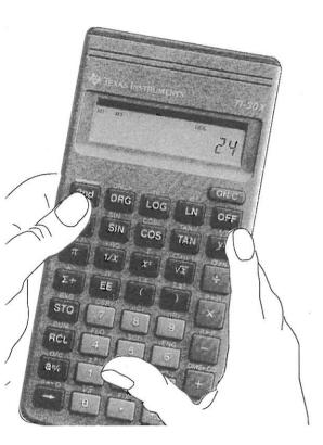
Calculation  $(1 + 2 + 3) \times 4 = 6 \times 4 = 24$ Key presses  $(1 + 2 + 3) \times 4 =$
