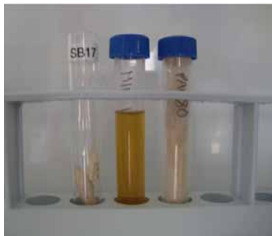
Figure 3. Extracting collagen, a protein, from archaeological bone samples. Most of the carbon in bone is stored in collagen. The extracted collagen is then combusted in a mass spectrometer to measure the relative proportions of its stable carbon isotopes.
