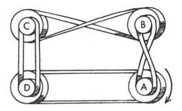
Four wheels are connected by belts. Two of the belts are crossed.
