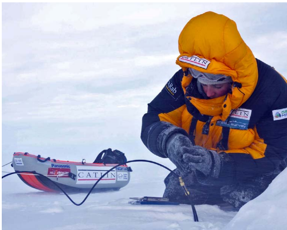
Dr. Helen Findlay measures the gas exchange through the sea ice between the air and ocean
