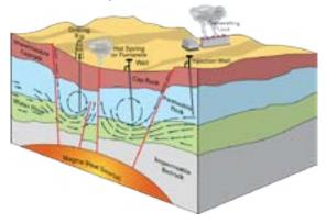
A geothermal power plant uses hot water or steam produced deep underground.
