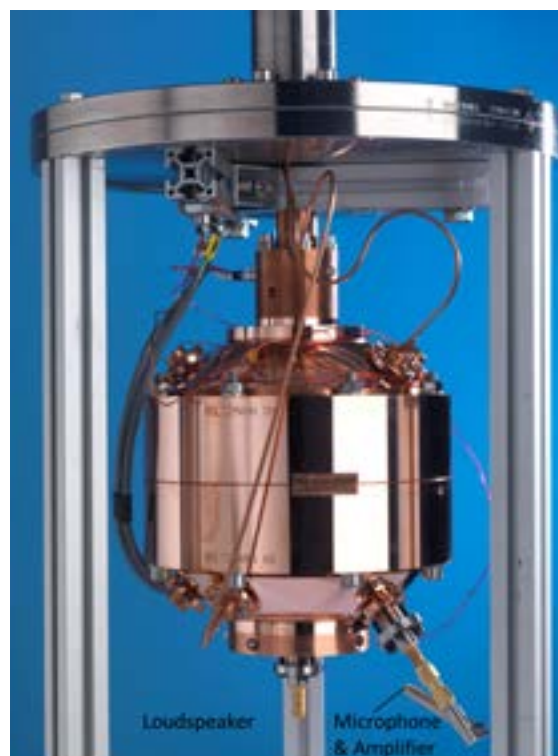
Our acoustic resonator is made from two hemispheres of copper which have been carefully machined and aligned to create an internal spherical hollow with a volume of approximately 1 litre.
