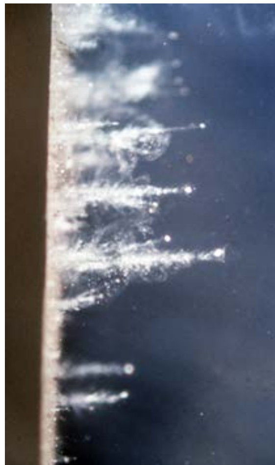
In a test of the material, particles were fired into a block of aerogel to mimic how comet dust will be captured in the Stardust mission.
