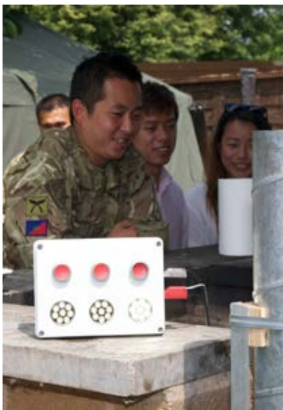
The Gurkhas cook lunch for their regiment on the stove to demonstrate how well it works. The electricity generated by the stove lights the LEDs.
