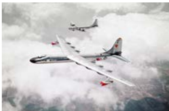
A nuclear test aircraft from the 1950s, carrying a thorium reactor. This is a USAF Convair Peacemaker, with a Boeing Superfortress beyond.
