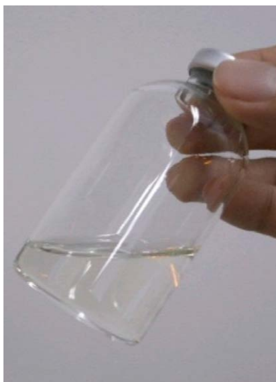
An ionic liquid (1-ethyl-3-methylimidazolium ethylsulfate; melting point < -20\text{ }^{\circ}\text{C} )
