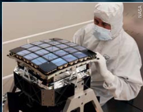
The array of CCDs which capture Kepler's images.
