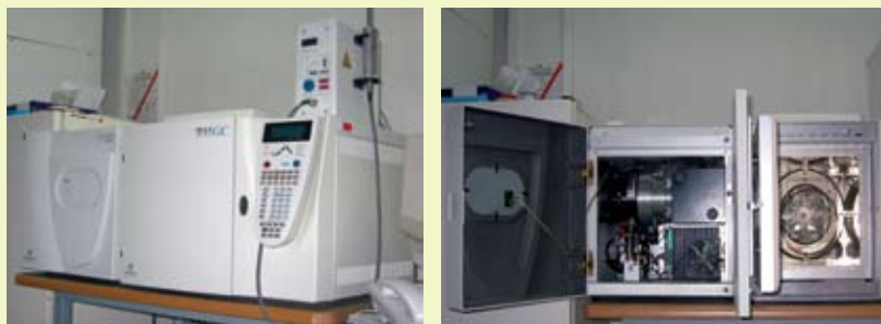
A GC-MS machine, closed and open. The chromatography takes place in the oven on the right; molecules are detected by the mass spectrometer on the left.
