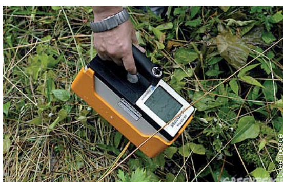
This type of radiation detector can tell which radioactive elements are present by measuring the exact energy of the gamma rays they emit.
