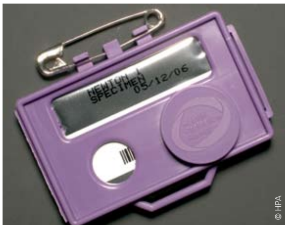
A film badge, worn by radiation workers, records their exposure to ionising radiation.
