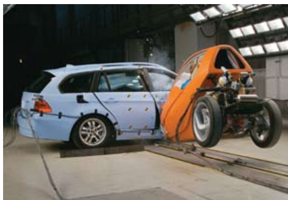
CLEVER undergoes a standard impact test in the EuroNCAP trials.
