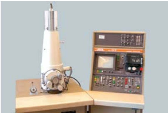
The tall microscope has controls to allow the operator to position the specimen in the electron beam. Images appear on the monitor screen.
