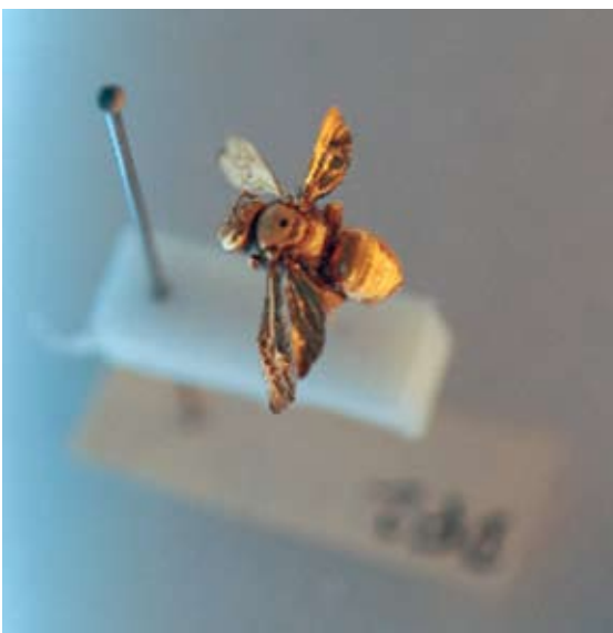
This bee has been coated with gold before being examined in an SEM.
