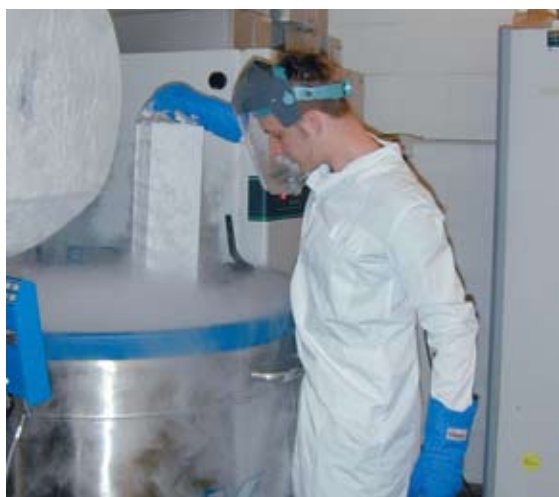
DNA samples are stored in liquid nitrogen at -196°C for future use.
