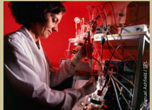
A researcher samples fluid from the artificial gut. The fluid will be tested to discover the chemical products of bacteria in the gut.
