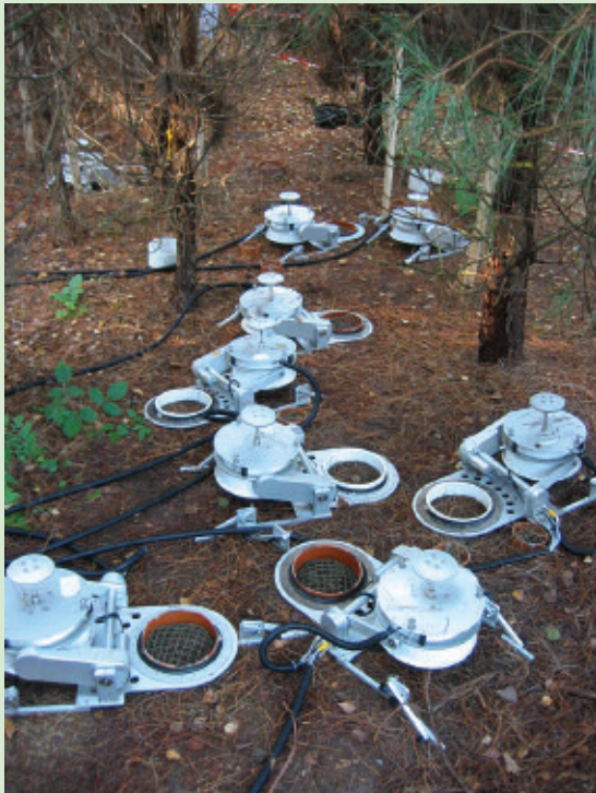
Above: Multiple chambers connected to a single IRGA in an 'Octopus' configuration
