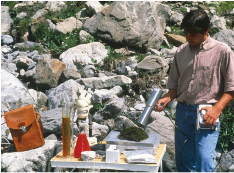
This scientist is using a Geiger counter to check moss samples collected from a mountainside
